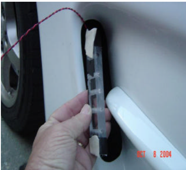
Foam Double Sided Tape in position
